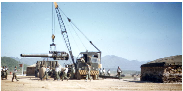
Disassembling a howitzer. The bunker to the right is where the powder and projectiles were housed. A crane was brought in when they moved a howitzer. A pit was dug by the crane for the trails and then the gun was mounted.
