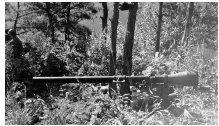
75mm recoilless rifle - shown while on reserve. It took four men to transport this weapon and the gunner carried the tripod and ammunition. This is the weapon Bob trained with and used in Korea, of which he said is why many men who used them now have hearing aids; the military had little if any ear protection back then. The gun used a perforated artillery shell casing, combined with a rear vented breech using propellant gases from the firing of a shell, to greatly reduce the recoil of the weapon.
