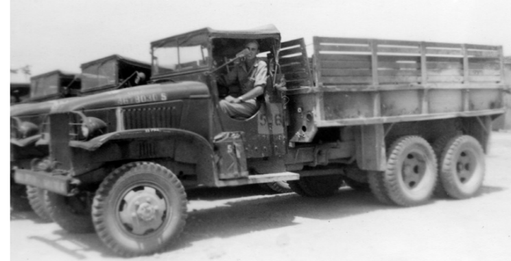
Duane in his truck - Because of the very high humidity, each night Duane had to drain the water from the air break tanks of his truck.
